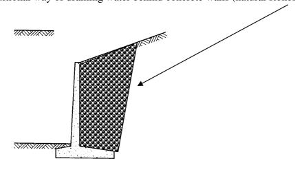
New way with draining panels filled with polystyrene "stones"
