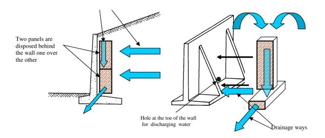
As you see in the section, 2 panels are installed behind a retaining wall one over other in order to obtain a "draining well" able to intercept water coming from slope and collect and discharge away.
