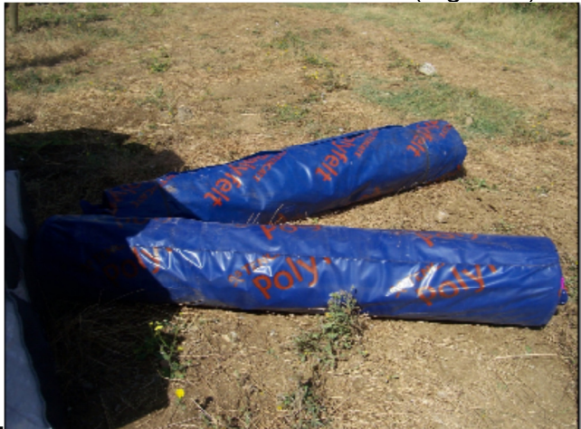
Figure 4 - Pieces of geotextile of the type non-woven fabric (TNT) used for cover IDROSAC 500 draining bags at the estate in Montalcino
